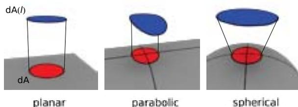
Fig. 6. Surface curvatures as area changes of parallel surfaces: Given a surface patch  $dA$ , the parallel patch is obtained by moving each point "off the surface" by a distance  $l$ . In doing so, the area changes as a polynomial  $dA(l) = dA(1 \pm lH + l^2K)$  defining two coefficients, called the mean curvature  $H$  and the Gaussian curvature  $K$ .
